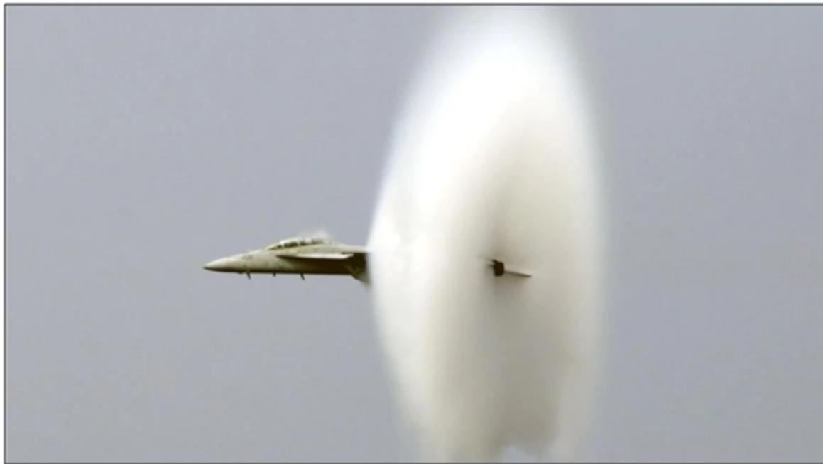
As this cone spreads across the landscape along the flight path, it creates a continuous sonic boom along the full width of the cone's base.
